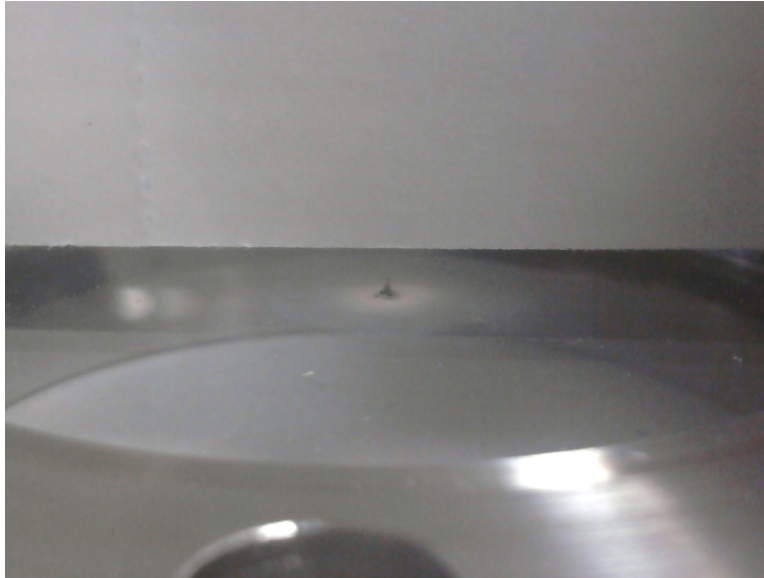
Figure 23. Visible rubidium accumulation (with an outer diameter of 1 cm with a raised cone in the center having a FWHM of approximately 0.05 cm ) on the calcium fluoride window closest to the exit of the capillary on the pump side chamber. The end of the tube was positioned about 1 cm away from the window and is shown in Figure 9. This validates rubidium successfully transferred through the 20 cm long, 500 \mu\text{m} inner-diameter capillary tube.
